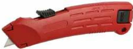
LAME AUTO-RÉTRACTABLE. OUVERTURE RAPIDE PAR PRESSION. CORPS ZAMAC. POUR TRAVAUX LOURDS. POIDS 200 G.
