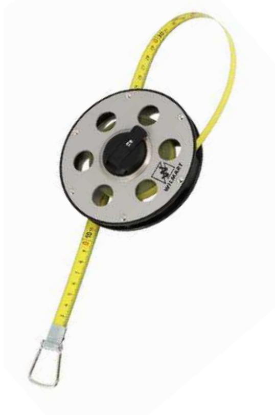
PROTECTION ABS SUR LA PÉRIPHÉRIE. BOÎTIER EN ALUMINIUM ANODISÉ. MANIVELLE ABS ESCAMOTABLE. RUBAN JAUNE ACIER LARGEUR 13 MM +FIBRE. LE 0 EST À LA BOUCLE CROCHET. LES OUVERTURES DANS LE BOÎTIER PERMET D'ÉVACUER FACILEMENT LES SALISSURES. GRADUATION EN MM UNIQUEMENT SUR LE BAS.
